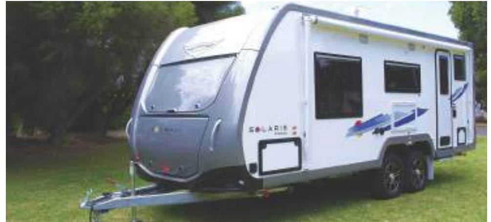
Composite walls, floor and roof provide excellent thermal and a acoustic insulation.
