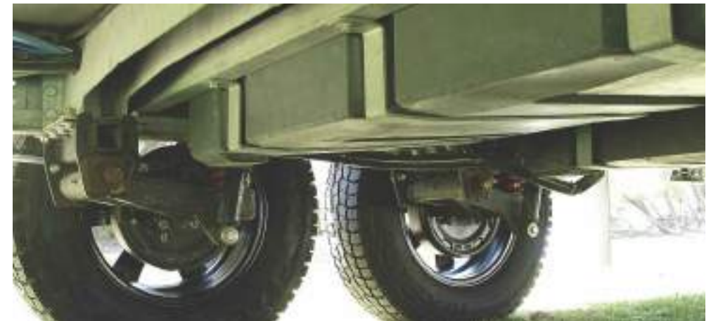
Trailing arm independent suspension and high ground clearance will get you more places
