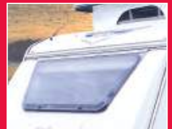
Double glazed windows for thermal & acoustic insulation
